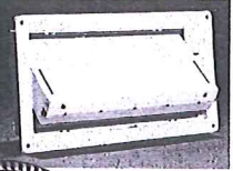
Float latch opens automatically in flood waters to equalize pressure and release flood waters.
